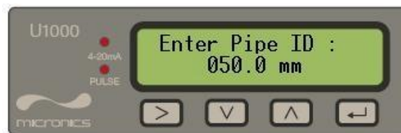
Figure 10 Enter Pipe ID Screen (Metric)
