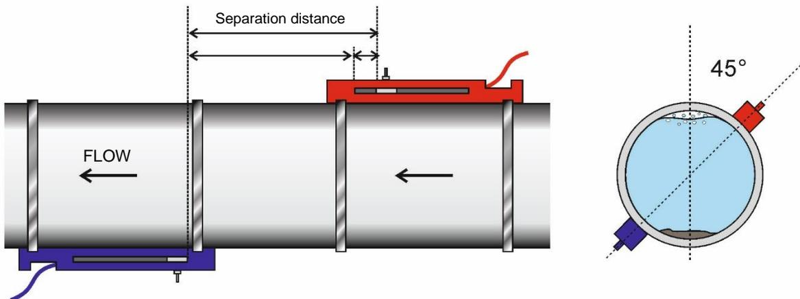
**Figure 18 Guide rail positioning for Diagonal Mode**
