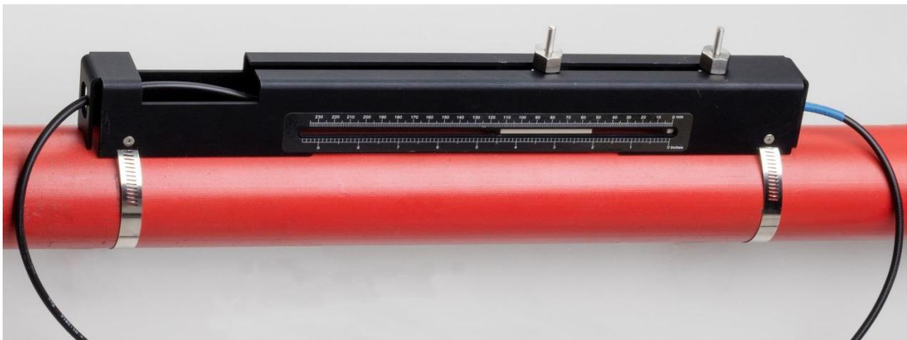
**Figure 17** Lowering transducers onto pipe
