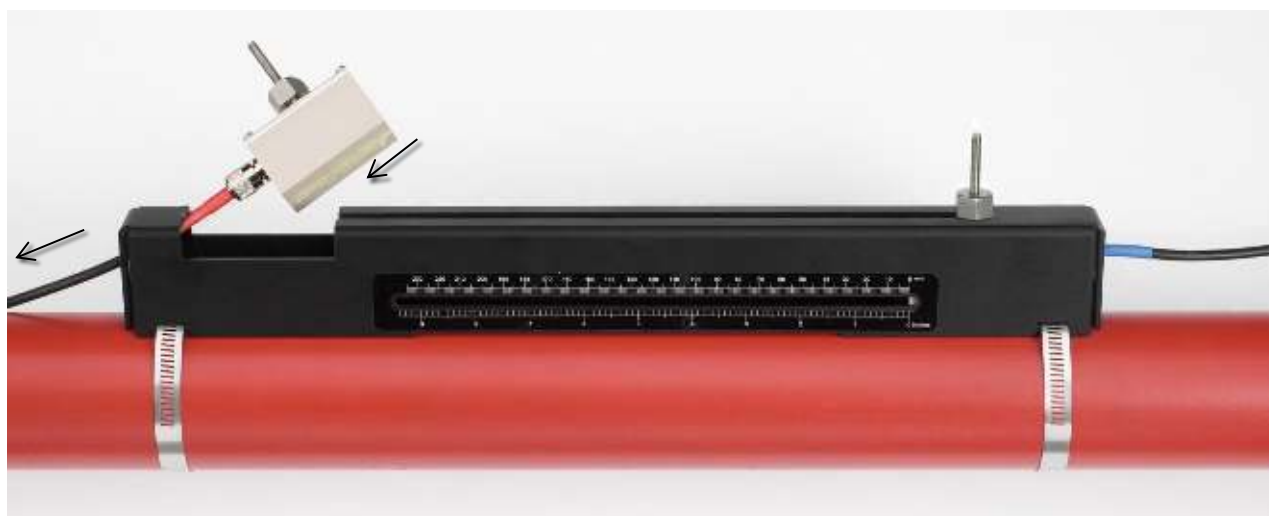
Figure 15 Installing upstream transducer (red)
