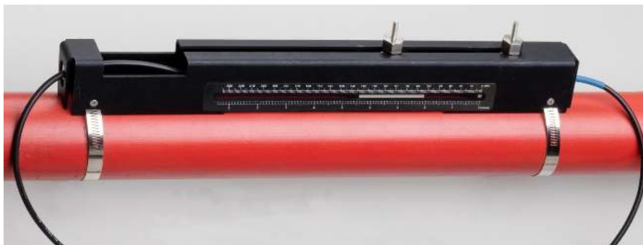
Figure 17 Lowering transducers onto pipe
