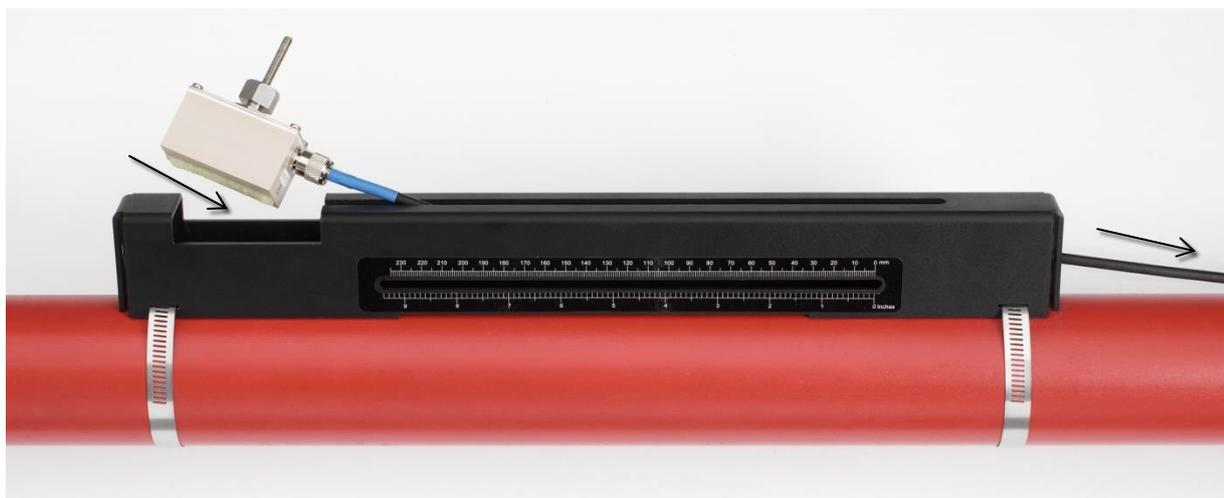
**Figure 13 Installing downstream (blue) transducer**
