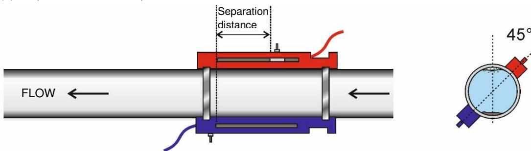
(b) Required transducer separation >230mm
