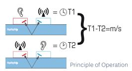
When ultrasound is transmitted between the transducers, its velocity is slightly increased when travelling in the direction of flow, and slightly reduced when travelling against the flow. The resulting transit time difference is directly proportional to the velocity of the flow in the pipe. Having measured the flow velocity and knowing the pipe cross-sectional area, the volumetric flow can be easily calculated.
