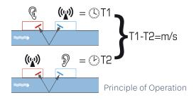
When ultrasound is transmitted between the transducers, its velocity is slightly increased when travelling in the direction of flow, and slightly reduced when travelling against the flow. The resulting transit time difference is directly proportional to the velocity of the flow in the pipe. Having measured the flow velocity and knowing the pipe cross–sectional area, the volumetric flow can be easily calculated.
