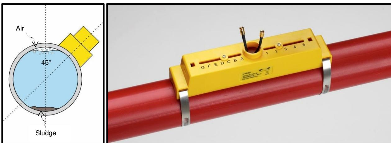
Sensor clamped at  $45^\circ$
